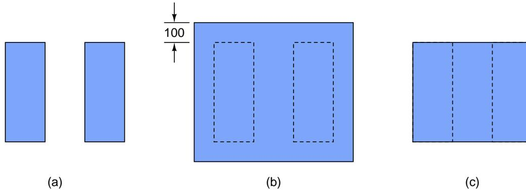
Figure 5: If the operator **grow 100** is applied to the shapes in (a), the merged shape in (b) results. If the operator **shrink 100** is applied to (b), the result is (c). However, if the two original shapes in (a) belong to different cells, and if CIF is generated separately in each cell, the result will be the same as in (a). Magic handles this by outputting additional information in the parent of the subcells to fill in the gap between the shapes.
