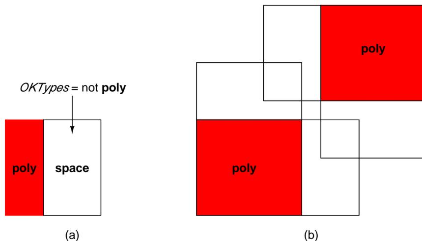
Figure 10: If only the simple rules from Figure 9 are used, errors may go unnoticed in corner regions. For example, the polysilicon spacing rule in (a) will fail to detect the error in (b).
