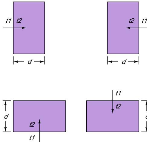
Figure 9: Design rules are applied at the edges between tiles in the same plane. A rule is specified in terms of type  $t1$  and type  $t2$ , the materials on either side of the edge. Each rule may be applied in any of four directions, as shown by the arrows. The simplest rules require that only certain mask types can appear within distance  $d$  on  $t2$ 's side of the edge.
