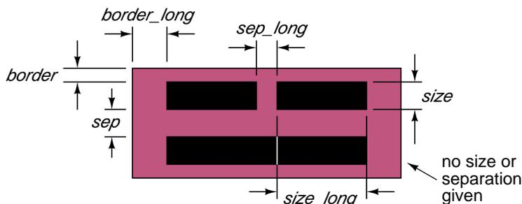
Figure 4: The **slots** operator chops each tile up into rectangles.
