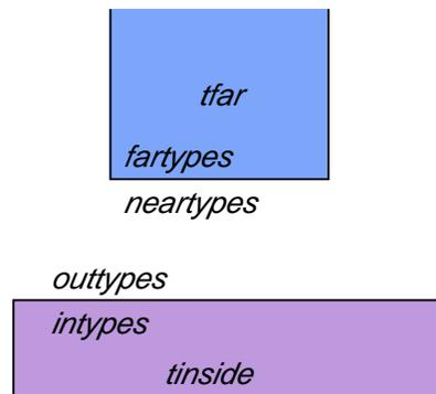
Figure 13: Parallel wire capacitance is between pairs of edges. The capacitance applies between the tiles *tinside* and *tfar* above, where *tinside*'s type is one of *intypes*, and *tfar*'s type is one of *fartypes*.
