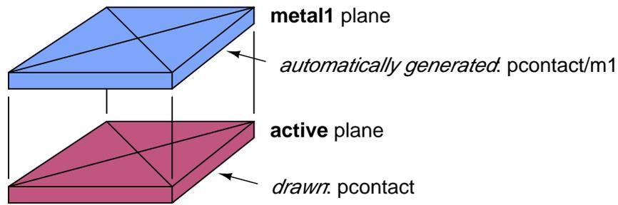
Figure 1: A different tile type is used to represent a contact on each plane that it connects. Here, a contact between poly on the **active** plane and metal1 on the **metal1** plane is stored as two tile types. One, **pcontact**, is specified in the technology file as residing on the **active** plane; the other is automatically-generated for the **metal1** plane.
