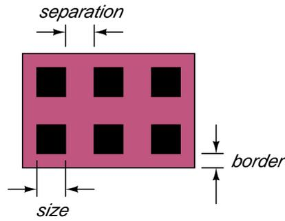
Figure 3: The **squares** operator chops each tile up into squares, as determined by the *border*, *size*, and *separation* parameters. In the example, the bold lines show the CIF that would be generated by a **squares** operation. The squares of material are always centered so that the borders on opposite sides are the same.
