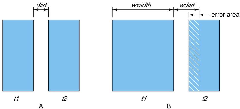
Figure 8: The **widespacing** rule covers situations like that shown above, in which material of type *t1* normally must be *dist* units away from type *t2* (situation A). However, if both dimensions of material type *t1* are larger than or equal to some width *wwidth* (situation B), then the spacing must be increased to *wdist*.
