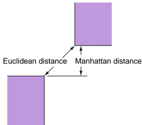
Figure 6: For design rule checking, the Manhattan distance between two horizontally or vertically aligned points is just the normal Euclidean distance. If they are not so aligned, then the Manhattan distance is the length of the longest side of the right triangle forming the diagonal line between the points.
