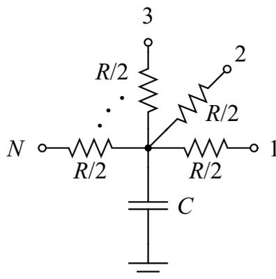
Figure 1: Each node extracted by Magic has a lumped resistance  $R$  and a lumped capacitance  $C$  to the substrate. These lumped values can be interpreted as in the diagram above, in which each device connected to the node is attached to one of the points  $1, 2, \dots, N$ .
