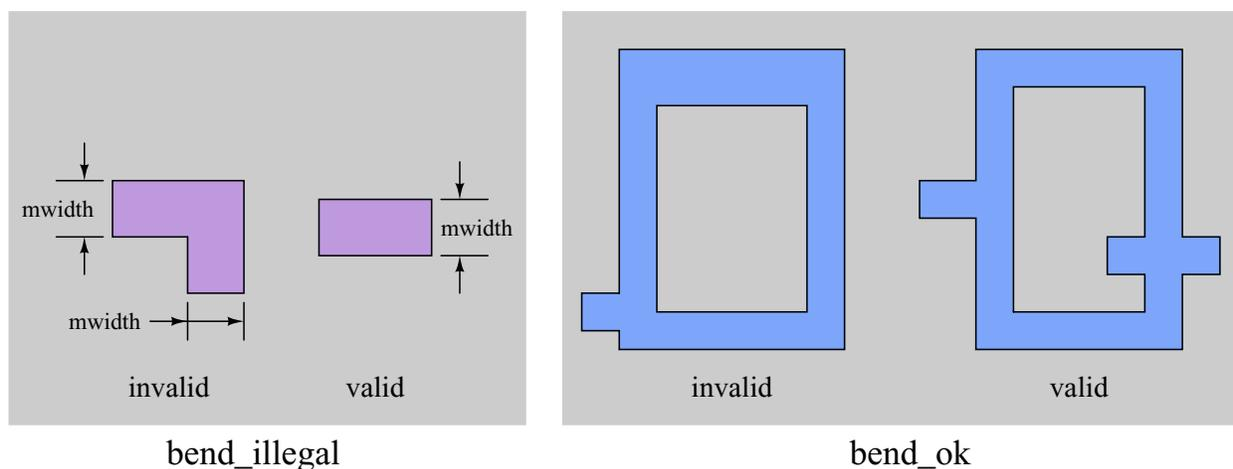
Figure 2: Examples of the maxwidth rule. The dogleg at the left would be ok in a **bend\_ok** rule, but fails in a **bend\_illegal** one, where the region's bounding box is checked. For **bend\_ok** rules, each tile in the region is checked. The left shape fails in two places: the top horizontal part is too thick and the stub at the bottom intersects the region in a shape other than a T or X.
